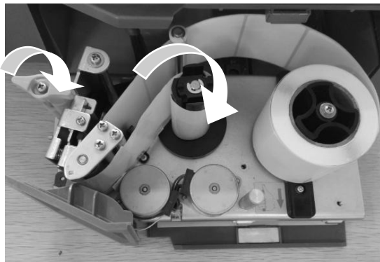
e. Thread the front of new label roll through the filter plate and wrap in pick-up clamp, and close the printing head (As shown in the figure)
